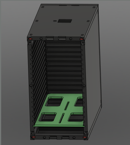
Fig. 5: Open SM with an installed slotcar tray.
